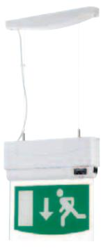
The wire suspension kit includes an adjustment device and clutch mechanism through which the wire is pulled until the desired length is reached. Excess wire can then be cut away. The cut end does not enter the first-fix plate so cannot chafe wiring or compromise safety.
