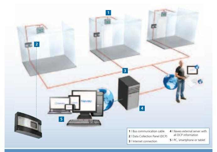
Each emergency lighting unit includes an individually addressed testing module which conducts functional and duration tests and communicates results to the DCP 2.
