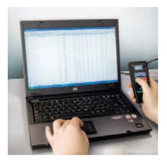
Testing can be done using the IR2-TX, 'test-only' transmitter, or the intelligent bi-directional handset (IR2-TESTWARE™ package), which tests, interrogates and reports. IR2-TESTWARE™ allows the user to view the results on small screen, or, as desired to download them to a PC to produce automated reports.
